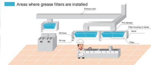
A grease filter is installed at the inlet of the exhaust duct in restaurant kitchens. It reduces grease build-up in the ducts and the risk of fire.
