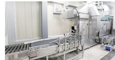
Automatic filter cleaning and drying with an automatically controlled crane
